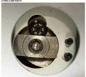
16.1.4. Use the 5mm Allen key to loosen the inner hexagon bolt (6) on the adjusting kit.
