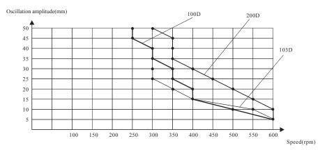
2.The adjustment of oscillation amplitude of ZHWY-103B multi-amplitude orbital constant temperature shaking incubator.
